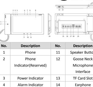
Speaker Button Goose Neck Microphone TF Card Slot Interface 5 Information Indicator 15 HDMI 6 Microphone 16 **USB** Interface 7 Camera 17 **Power Interface** 8 Screen Terminals 18 9 Answer/Hang Up 19 Network Interface Button 10 **Unlock Button**
